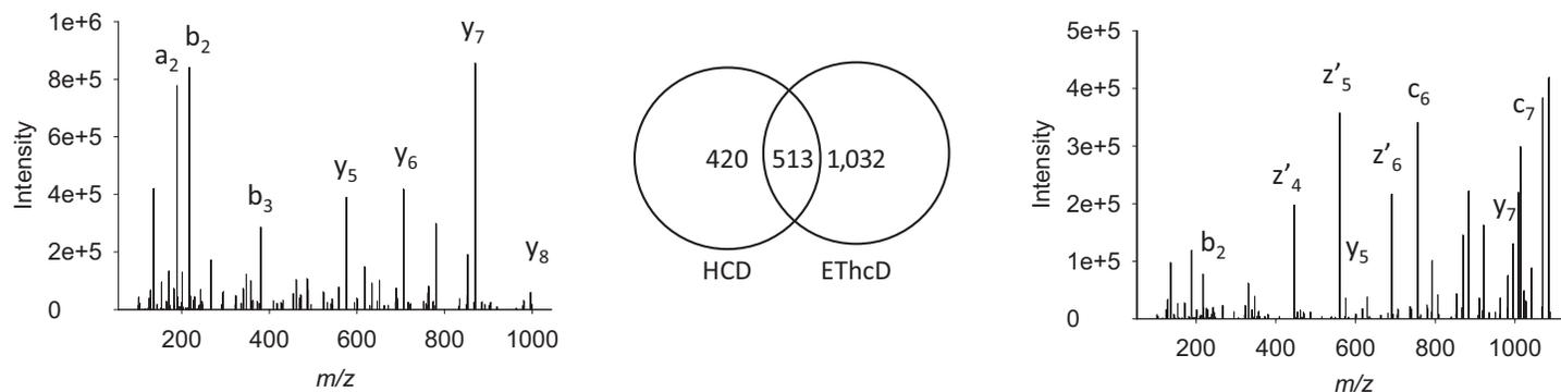
**Figure 4. HCD versus EThcD:** HCD (note b and y ions) and EThcD (note b, y, c, and z ions) spectra of the peptide SEYMNN-KEA. The Venn diagram shows the number of unique peptides acquired from a single sample using both approaches.
