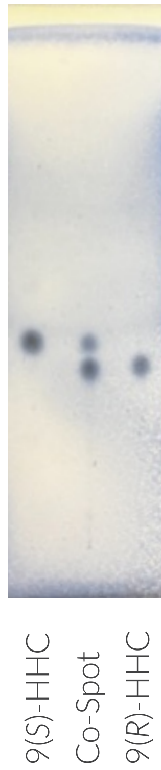
FIGURE 3 – TLC of 9(S)- and 9(R)-HHC on silica gel developed with 10% MTBE in heptane and visualized by ceric ammonium molybdate (CAM)
